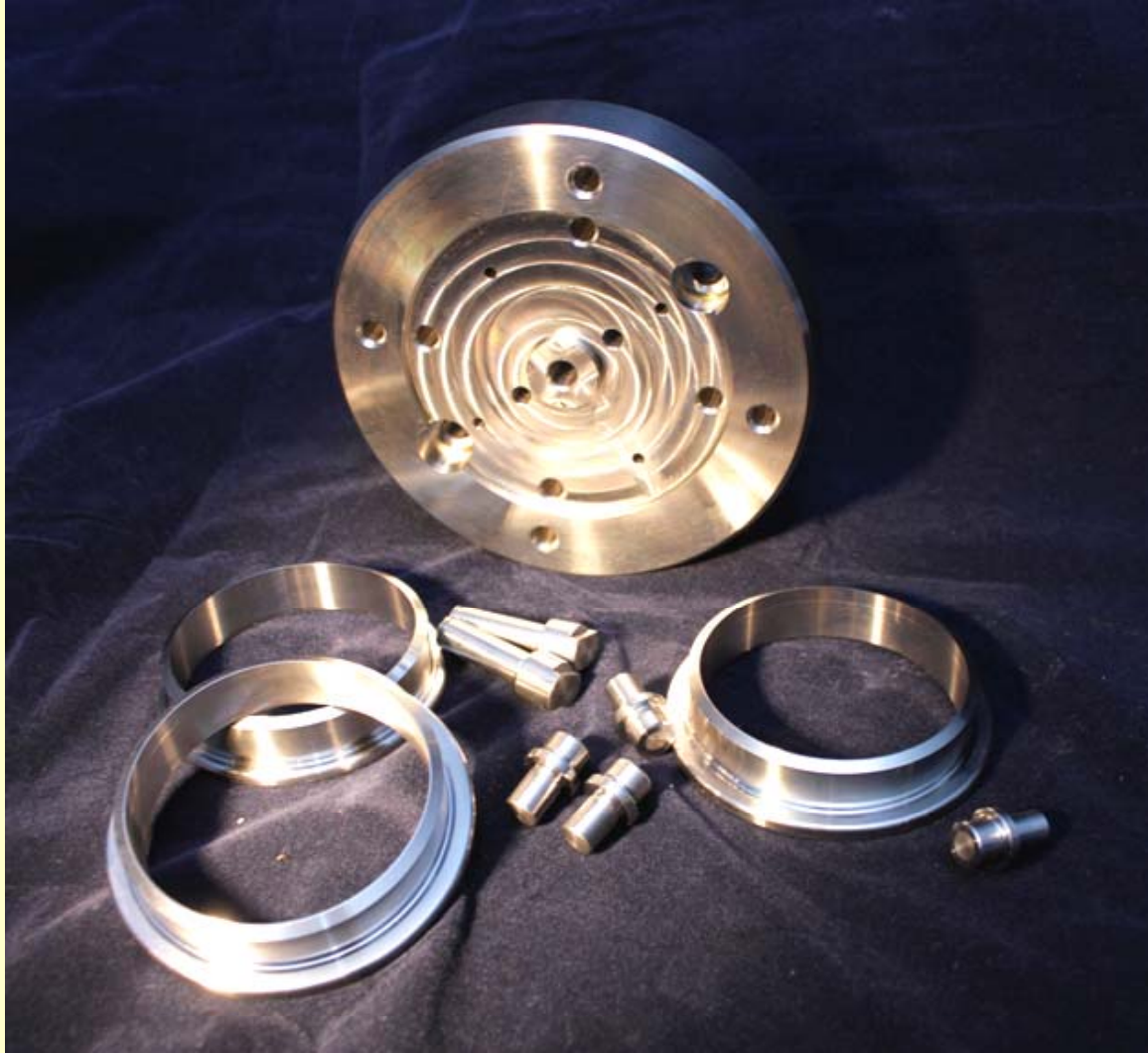
CNC Turning Parts
